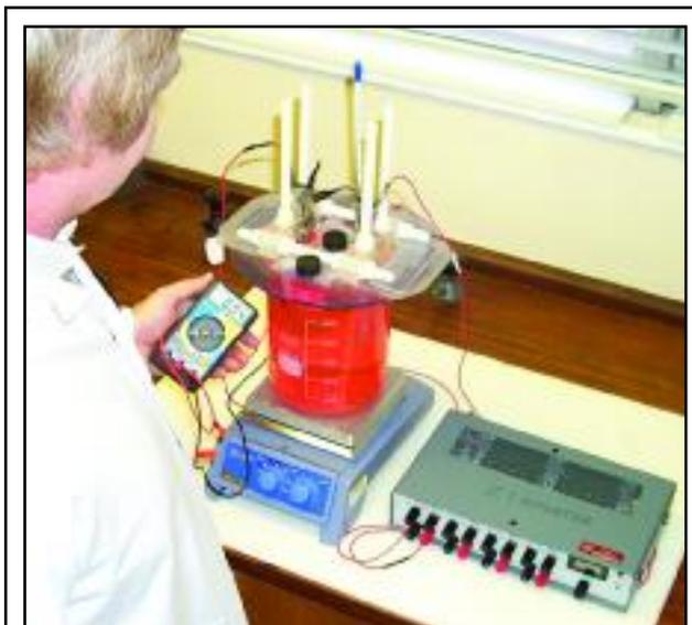
Apparatus has been built at TARRC to test hose samples for electrochemical degradation, the primary cause of automotive coolant hose. The apparatus includes the use of a zero impedance ammeter, which is providing better insights through more consistent measurements of very low current flows. The knowledge gained is enabling ideas of the detailed mechanisms operating in ECD.
