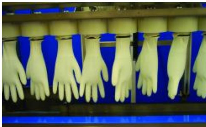
*Testing gloves for holes using the condom electronic leak tester developed at TARRC is far more efficient in terms of time and manpower than the water leak test in the glove Standard. This equipment could be readily adapted to perform the rapid screening of gloves for holes.*
