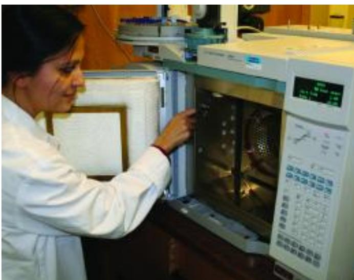
*Rubber Consultants continues to generate a major part of its income from analysis, particularly for the pharmaceutical industry. A new capillary column is fitted to a GC-MS prior to analysing pharmaceutical samples.*
